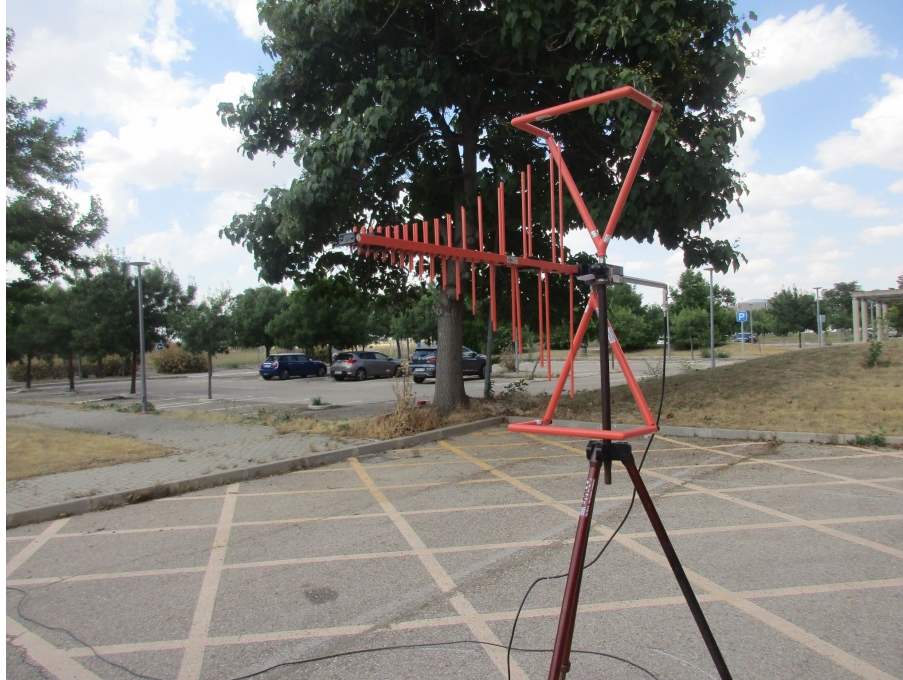
Figure 13: CBL6143A antenna (Schaffner) used for gain calibration
