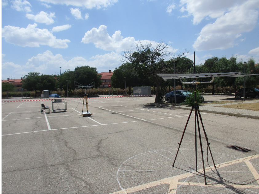
Figure 7: Radiation pattern. Test setup. Horizontal Polarized Mount (E-Plane)
