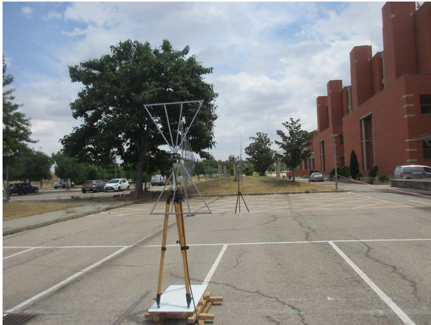
Figure 8: Radiation pattern. Test setup. Vertical Polarized Mount (H-Plane)
