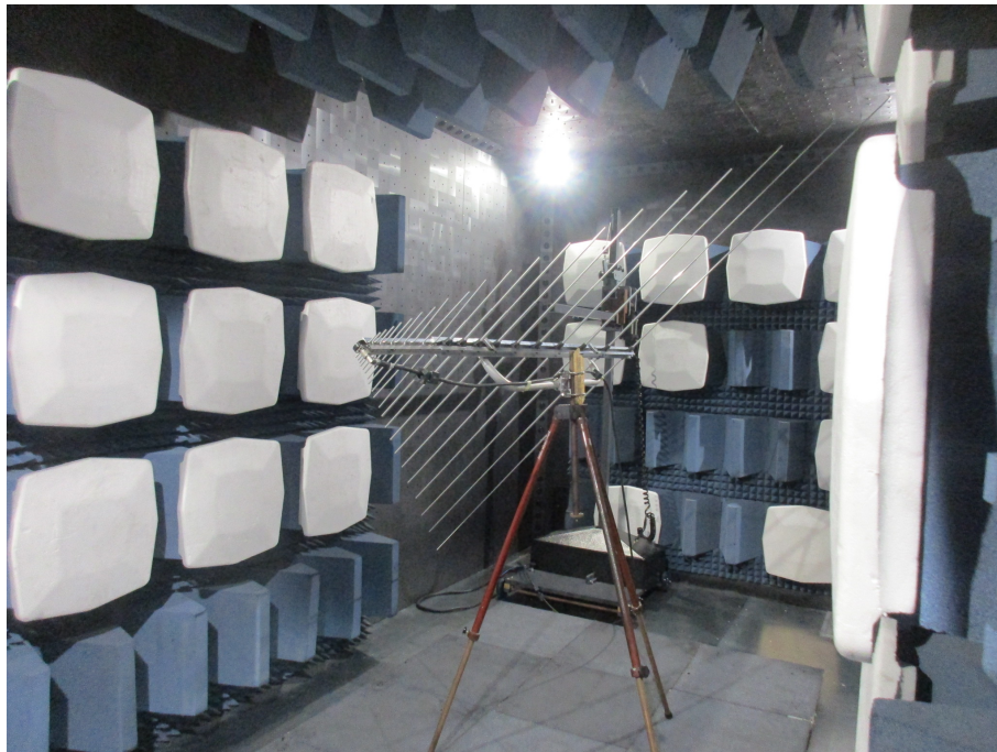
Figure 3: CLP-5130-1N inside the chamber
