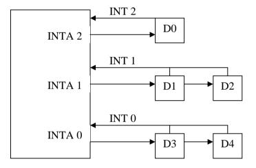
D1 and D2 and D3 and D4 are respectively daisy chain attached.
