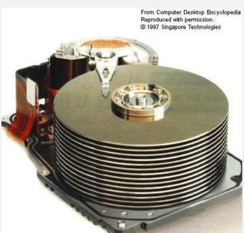
Figure: Magnetic disc (Pic: img.zdnet.com)
