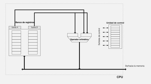
Figure: CPU internal structure
