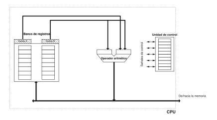
Figure: CPU internal structure
