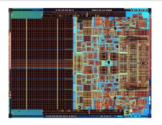
Figure: Intel Core Duo Processor (Pic: www.linuxhardware.org)
