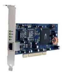
Figure: Ethernet board (Pic: cache.gizmodo.com)
